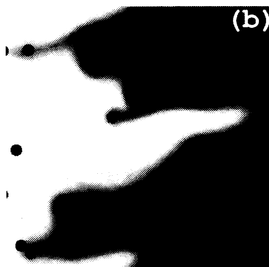
Fig. 4. Examples of dispersion through porous media in the limit where the pore space is near its percolation threshold (panel a) and in the opposite limit where the solid fraction is only 5 percent (panel b).
